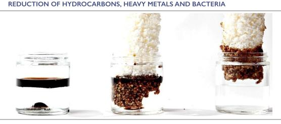
AbTech Industries' Smart Sponge technology is at the heart of its product innovation. Smart Sponge's unique molecular structure is based on innovative polymer technologies that are chemically selective to hydrocarbons. Certain variations of the media can reduce bacteria levels (Plus) and remove heavy metals (HM). Products incorporating Smart Sponge technology are non-mechanical, do not require structural changes to stormwater systems and are easily installed and maintained.
